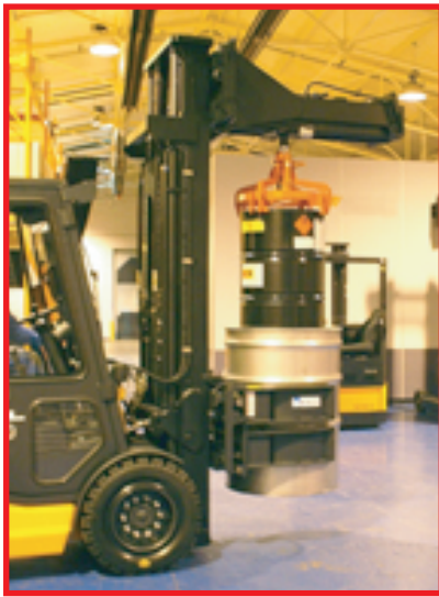
B&B Attachments specially designed the rig for retrieval and repacking of drums at BNFL.
